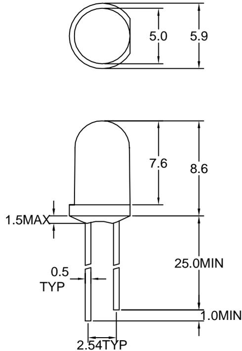
Note : 1.All dimension are in millimeter tolerance is  $\pm 0.25$ mm unless otherwise noted.
